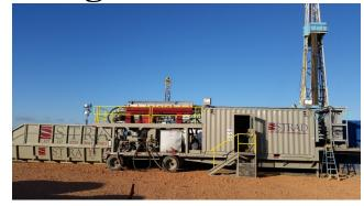
transported trailer that can be up and running within 60 minutes of arriving on site. This plug and play design significantly reduces rig up costs and does not require crane assistance in order to be begin the solids control process.
